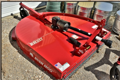
BUSH HOG BH317 Rotary Cutter, single spindle, 84" cutting width, 50 HP PTO min., 10-yr. gearbox lim. warr., 2' cutting diameter..... $4,480 $3,680
