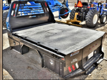
BESLER 9102SK Flatbed—Single wheel, long bed, 56" cab to axle, four tool boxes..... $3,990 $3,490
